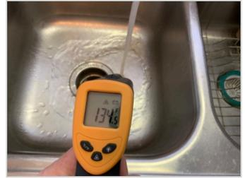
**The hot water temperature was greater than 125F and may pose a risk of burning.** HomeTeam recommends adjusting the hot water temperature by turning down the water heater thermostat.
